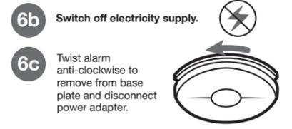
**6c** Twist alarm anti-clockwise to remove from base plate and disconnect power adapter.
