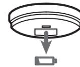
**6e** Always test the alarm after replacing the batteries.
