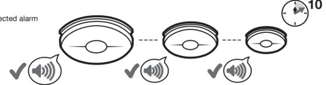
On an interconnected network, only the alarm that senses the fire will sound and flash its LED. Other connected alarms will sound a warning but will not flash their LED. Do not connect more than 11 other devices.
