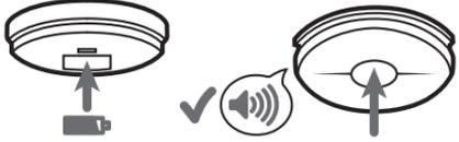
**2c** Push and twist the alarm clockwise onto the base plate. Turn the electricity supply back on and check that the green LED is on.
