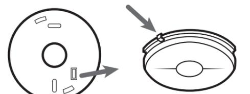
To enable removal of the alarm, withdraw the locking plug with a pair of pliers.
